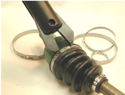
Pneumatic tool for closing Oetiker hose clamps. (Right, below)
